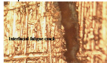
Fatigue crack propagation
