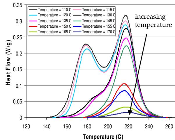
Subsequent DSC scan data at 10 °C/min of samples cured isothermally at the temperatures shown in the legend box (Exposure dose = 2000 mJ/cm<sup>2</sup>)
